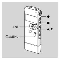
You can set the VOR (Voice Operated Recording) function to "ON," to make the IC recorder start recording when the IC recorder detects sound, and pause when no sound is heard, eliminating recording during soundless periods.
